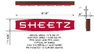
CANOPY MOUNTED SHEETZ SIGN DETAIL SCALE: 1/2" = 1'-0"
