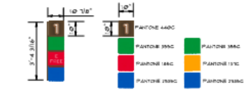
DOUBLE FACED FUEL OFFERING FLAG SIGN DETAILS SCALE 1/2" = 1'-0"
